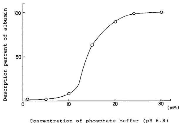
Fig. 2. Desorption ratio of proteins on hydroxyapatite column. Column, 50 mm  $\times$  4.5 mm I.D.; flow-rate, 0.8 ml/min; UV detector, 280 nm; sample, control serum; sample volume, 2  $\mu$ l. Serum globulin is desorbed with 100 mM phosphate buffer (pH 6.8).
