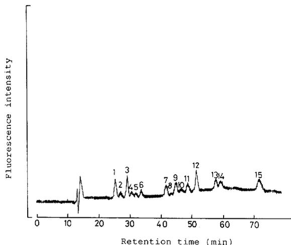
Fig. 6. Typical chromatogram of a normal human serum (male; age 63). Chromatographic conditions as in Fig. 5. Peaks: 1=GUDCA; 2=TUDCA; 3=UDCA; 4=GCA; 5=TCA; 6=CA; 7=GCDCA; 8=TCDC; 9=GDCA; 10=TDCA; 11=CDCA; 12=DCA; 13=GLCA; 14=TLCA; 15=LCA. Sample volume, 40  $\mu$ l.
